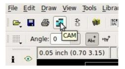
In Eagle, open Board view. Click the "CAM" button or choose "File->CAM Processor". This will open the CAM Processor tool that is used to generate the files.
